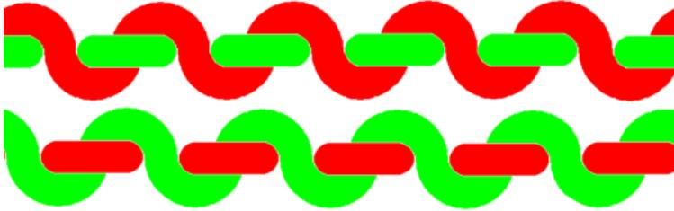
Figure 3: Top and Side Views of Braided Wires
