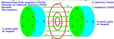
A changing magnetic flux through a circular area generates a loop electric field which accelerates the electrons in a Betatron. Green is transformed into red.
